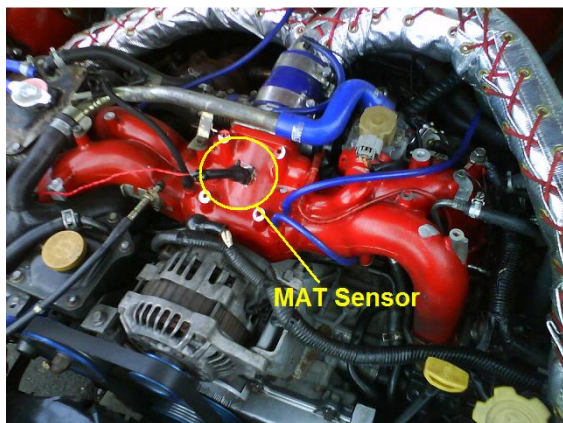
Figure 20 - MAT sensor location
