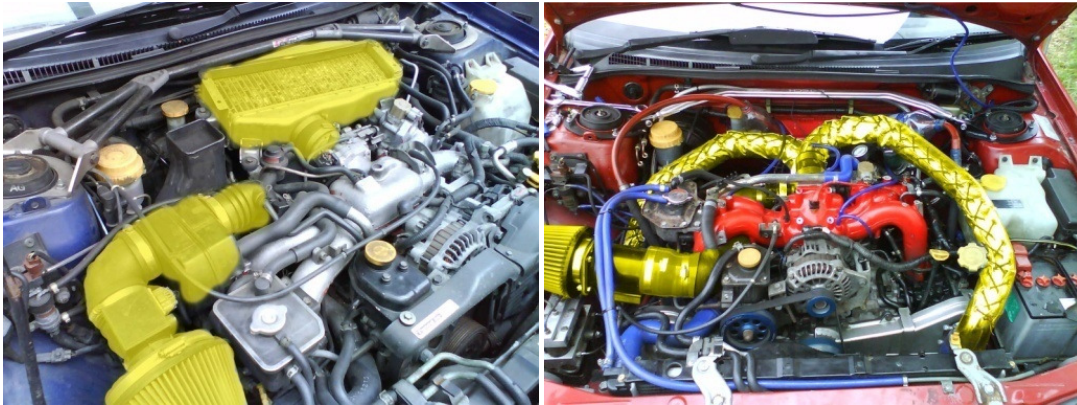
Figure 2 - Standard air duct route (left) and front mounted intercooler air duct route (right). Highlighted in yellow. (Photographed by author)
